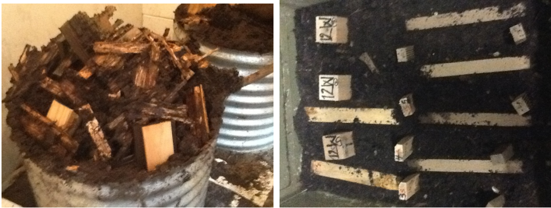
Figure 4: Wood plastic and P. radiata test blocks exposed to termite colony (left) and decay fungi (right).
