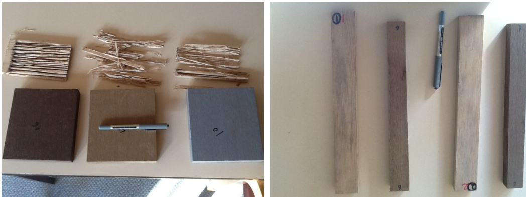
Figure 5: Wood plastic and radiata pine samples after eight weeks exposure to termites (left) and twelve weeks exposure to decay fungi (right).
