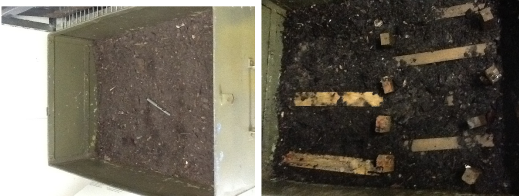
Figure 2: Decay test tank (1200 L X 750 W X 750 D mm) with freshly collected soil and test stakes installed in-ground and above ground on the soil surface exposure.
